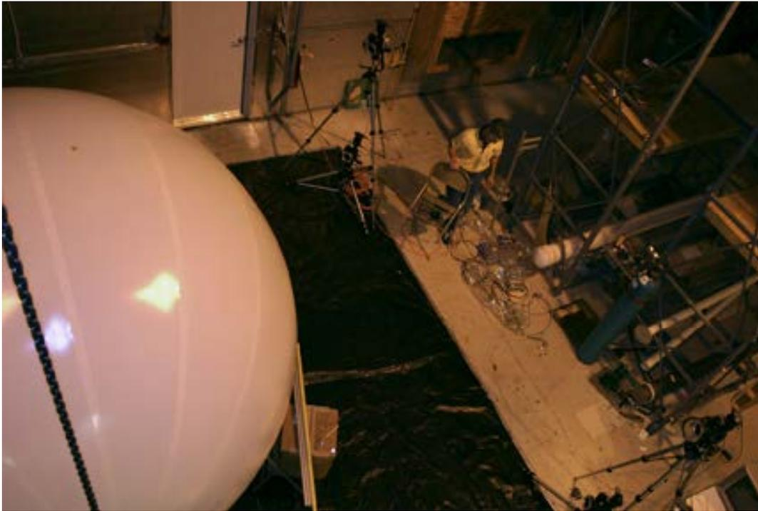
**Figure 9. Camera positions with respect to the balloon.**
