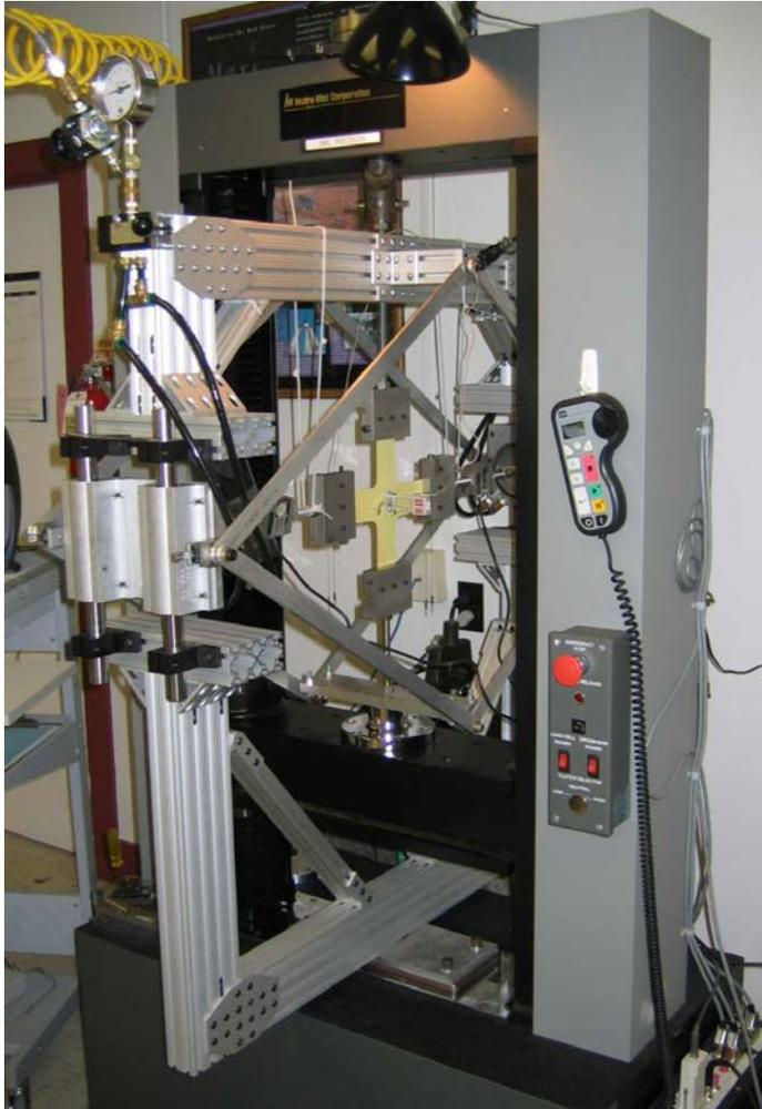
**Figure 5. Bi-axial test device installed in Instron.**
