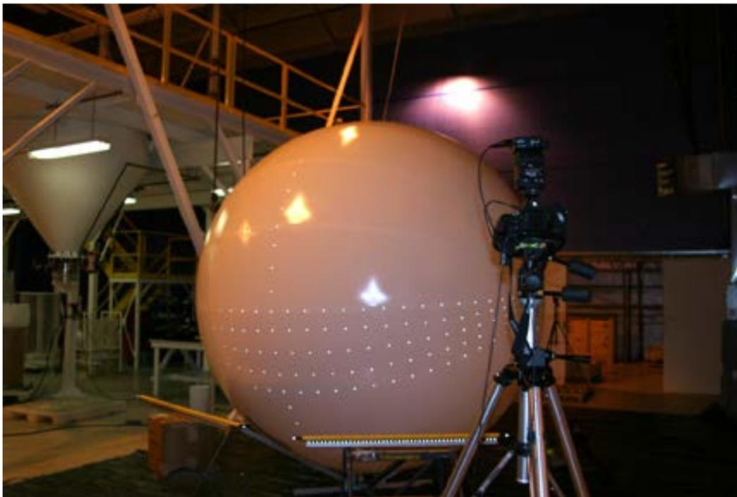
Figure 8. Balloon with retro-reflective targets.
