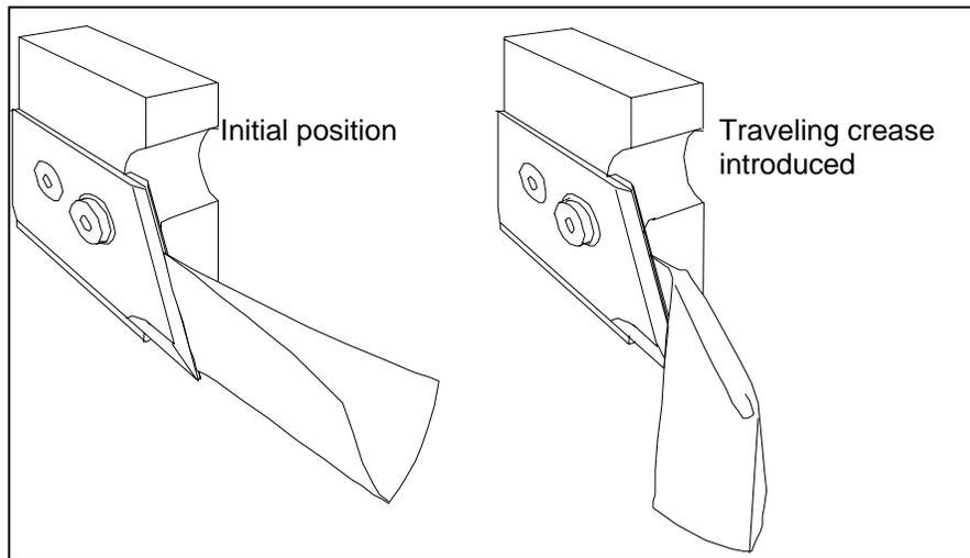
**Figure 7. Specimen Set Up of ASTM D 6182 Bally Flexometer**
