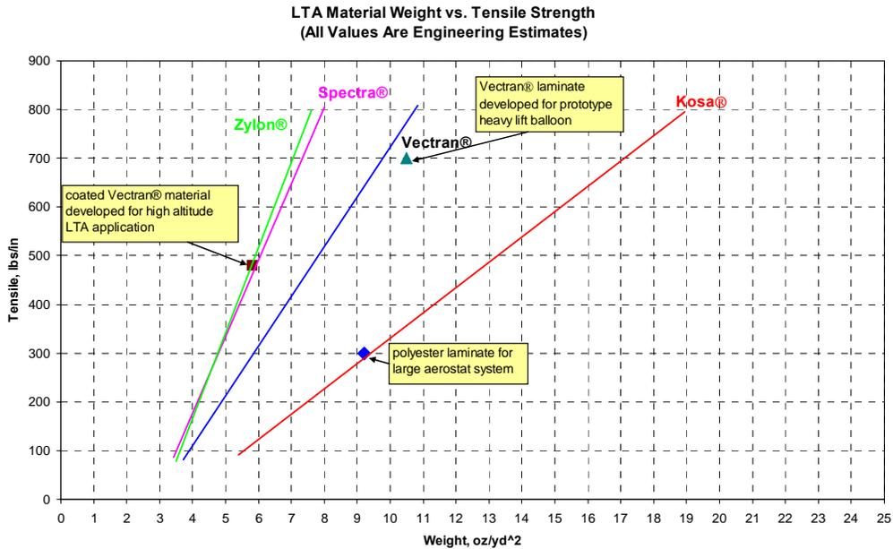
**Figure 5. Theoretical Weight vs. Strength for Laminated LTA Material**
