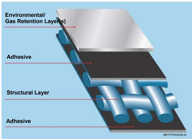
**Figure 2. Typical Hull Material Layout**
