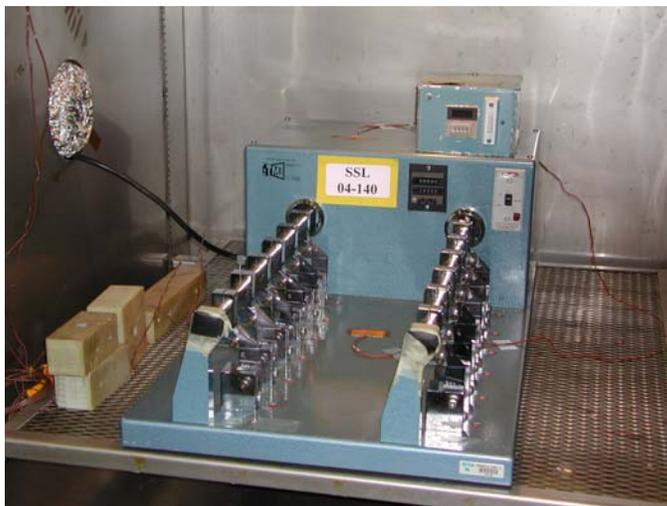
**Figure 8. Bally Flexometer in a Cold Chamber**
