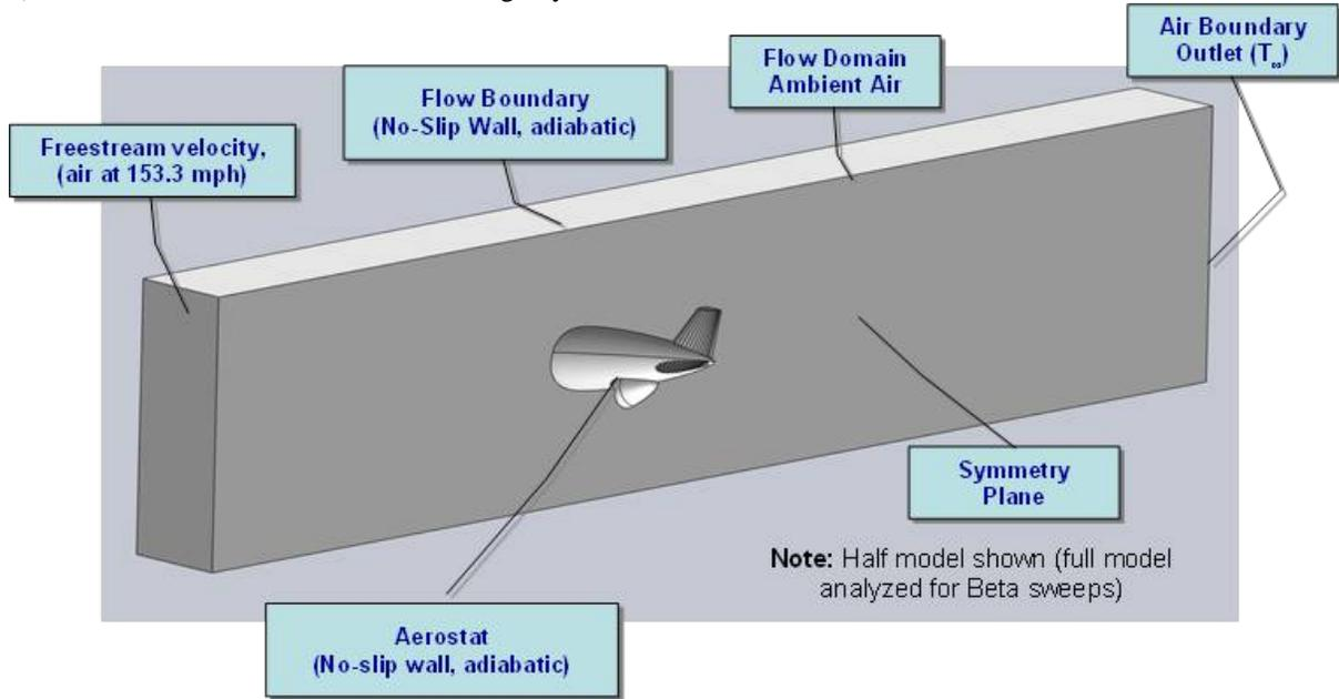
**Figure 2. CFD boundary conditions**
