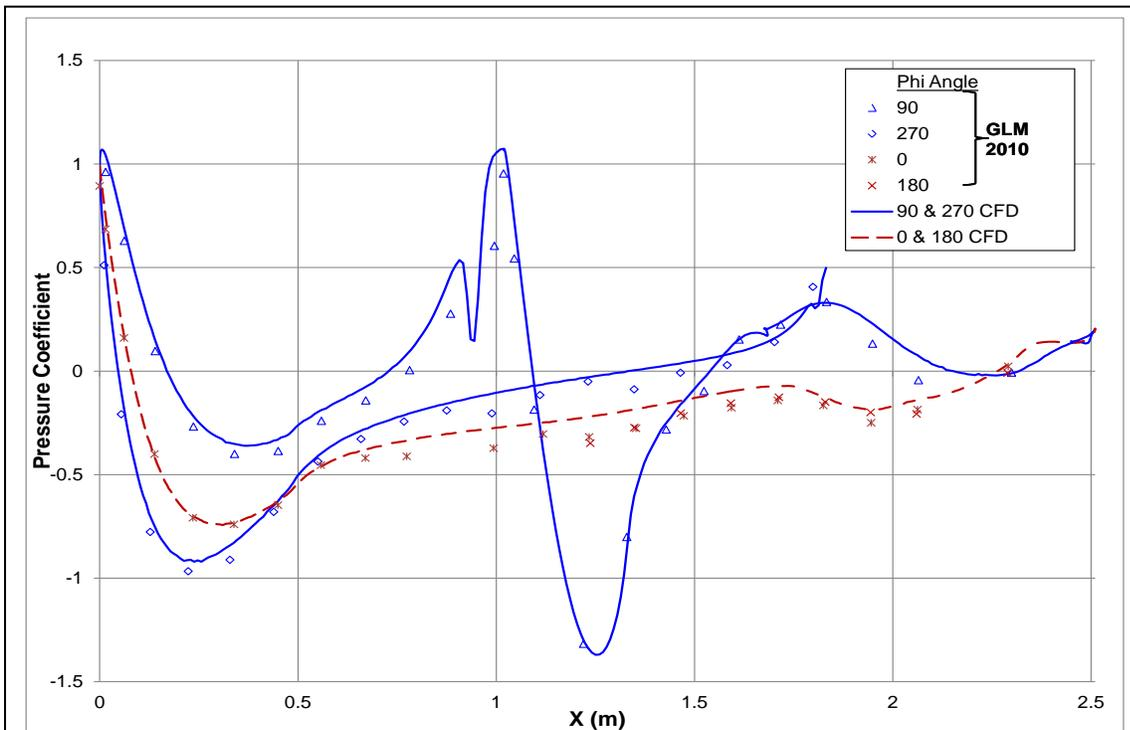
Figure 7 Pressure Comparison for 10 Deg. Pitch and Zero Yaw.
